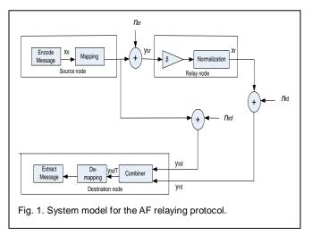
The source node broadcast its signal to both the relay as well as the destination node in the first time slot. The signal is received at both the relay node and the destination node. The received signal at the relay  $y_{av}$  as well as the destination nodes  $y_{ad}$  as given by [2],[16]
