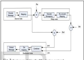
Fig. 2. System model for the DF relaying protocol.
